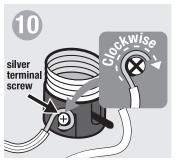
Wrap each wire clockwise 3/4 turn under head of terminal screw. Tighten screws. Cut loose strands.
