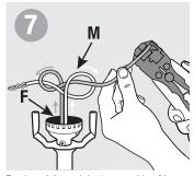
Feed cord through bottom or side of lamp, up through nipple and out socket cap (F). Split cord about 2" from end and tie an Underwriter's Knot (M).
