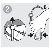
Lift sleeves (L) toward top and gently squeeze harp (B) sides. Remove from harp bottom (H).
