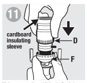
Make sure cardboard lining is firmly in place in socket shell (D). Place socket shell on cap (F). Pull extra wire back through lamp. Snap socket shell into socket cap by gently rocking side-to-side, until shell snaps into place with a clicking sound.
