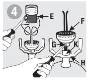
Unscrew terminal screws (E) to release wires. Unscrew socket screw (G). Unscrew socket cap (F) from lamp nipple (K) and remove. Remove harp bottom (H). Pull cord through bottom or side of fixture to remove.
