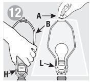
Insert top of harp (B) into harp bottom (H) and slide sleeves (L) to lock in place. Insert bulb, shade and finial (A).
