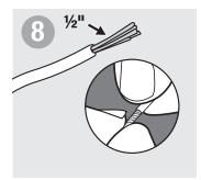
Using wire stripper, expose ½" of bare copper strands from cord. Twist copper strands tightly together.
