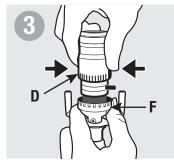
Press sides of socket shell (D); rock shell back and forth and lift up to remove from socket cap (F).
