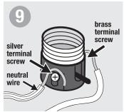
Connect ribbed neutral wire (feel outside of cord for ribbing) around silver terminal screw and smooth wire around brass terminal screw.
