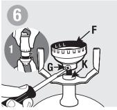
Remove socket cap from socket shell and loosen socket screw (1). Thread socket cap (F) onto lamp nipple (K) and tighten. Tighten socket screw (G). Cardboard insulation disc should be firmly in bottom of socket cap.
