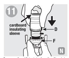
Ensure cardboard lining is in place, then fit socket shell (D) into socket cap (F) by gently rocking side-to-side, until shell snaps into place with clicking sound.
