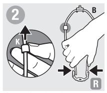
Lift sleeves (K) toward top and gently squeeze harp (B) sides. Remove from harp bottom (H).
