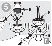
Unscrew terminal screws (E) to release wires. Unscrew socket screw (G). Unscrew socket cap (F) from lamp nipple (J) and remove. Remove harp bottom (H).
