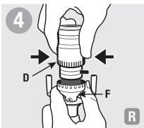
Press sides of socket shell (D); rock shell back and forth and lift up to remove from socket cap (F).
