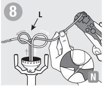
Split cord about 2" from end and tie an Underwriter's Knot (L). Using a wire stripper, expose 1/2" of bare copper strands from cord. Twist copper strands tightly together.
