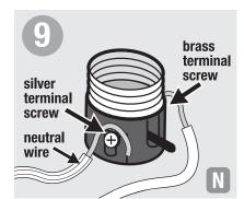
Connect ribbed neutral wire (feel outside of cord for ribbing) around silver terminal screw. If no ribbing, determine the neutral wire and connect around silver terminal screw. Connect smooth wire around brass terminal screw.
