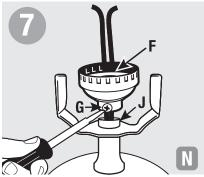
Insert wires through bottom of socket cap (F). Thread socket cap onto lamp nipple (J) and tighten. Tighten socket screw (G). Cardboard insulation disc should be firmly in bottom of socket cap (F).
