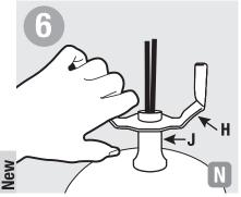
Place new harp bottom (H) over lamp nipple (J) and feed wires through.
