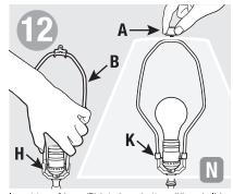
Insert top of harp (B) into harp bottom (H) and slide sleeves (K) to lock in place. Insert bulb, shade and finial (A).
