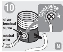
Wrap each wire clockwise 3/4 turn under head of terminal screw. Tighten screws. Cut loose strands.
