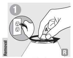
Before beginning **TURN OFF POWER** by unplugging lamp from wall outlet. Unscrew finial (A), remove lamp shade and bulb.
