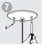
Cover with canopy and secure with mounting screws (E).
