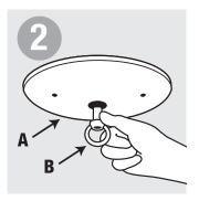
Insert loop (B) into hole from outside of canopy (A).
