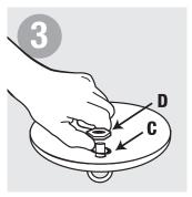
Secure from inside of canopy with washer (C) followed by nut (D). Tighten.
