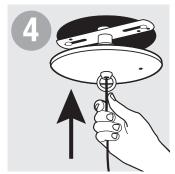
Pass wires from fixture up through hole in loop to inside of canopy.
