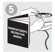
While supporting the fixture, attach wires to according to manufacturer's instructions.
